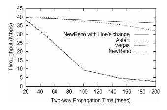
Figure 11. Throughput vs. two-way propagation time (first 20 seconds)
