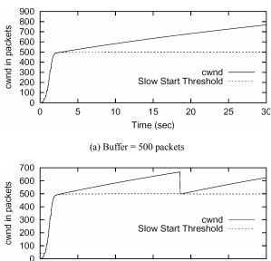
Figure 5. Astart cwnd dynamic during startup phase (Bottleneck bandwidth =40 Mbps, RTT=100ms, BDP =500 packets,)
