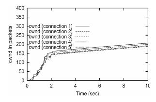
Figure 7. Astart cwnd Dynamic when 5 connections start at the same time (Bottleneck Bandwidth=40Mbps, RTT=100ms, BDP=500 packets)
