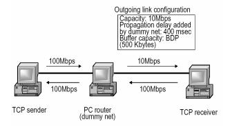
Figure 16. Measurement topology and configuration
