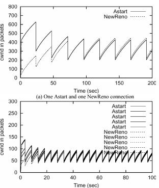
(b) Five Astart and five NewReno connections Figure 13. *cwnd* dynamics between Astart and NewReno (Bottlneck band width is 50Mbps, and RTT is 70msec)
