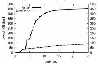
Figure 17. cwnd dynamics in Astart and NewReno at Start-up (Lab Measurements Results)
