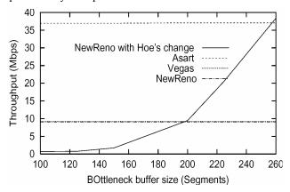
Figure 10. Throughput vs. bottleneck buffer size (first 20 seconds)
