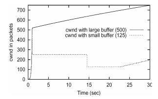
Figure 3. cwnd dynamics in NewReno with Hoe's modification
