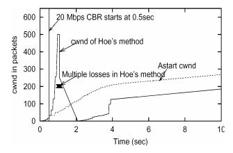
Figure 8. cwnd Dynamic with UDP traffic joins in during srartup(Bottleneck capacity=40 Mbps, RTT=100ms, BDP =500 packets)
