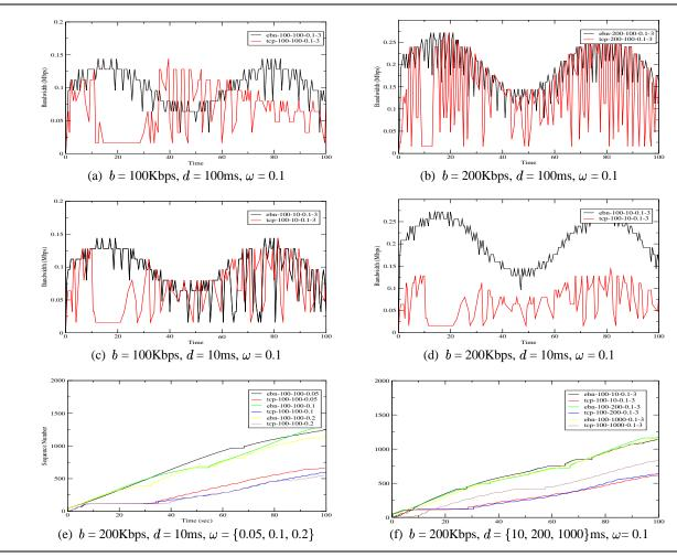
Fig. 3. Comparisons between TCP-EBN and TCP-NewReno ( $\alpha = 3$ )
