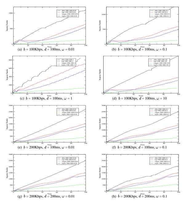
Fig. 4. Comparisons between TCP-EBN, TCP-NewReno, TCP-Vegas, and TCP-Westwood
