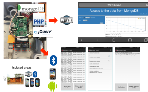
Figure 8: Fully autonomous LoRa gateway
