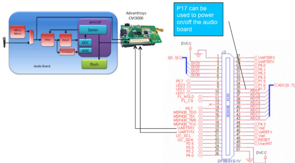
Figure 11: developed audio board connectivity schema on an Advanticsys TelosB
