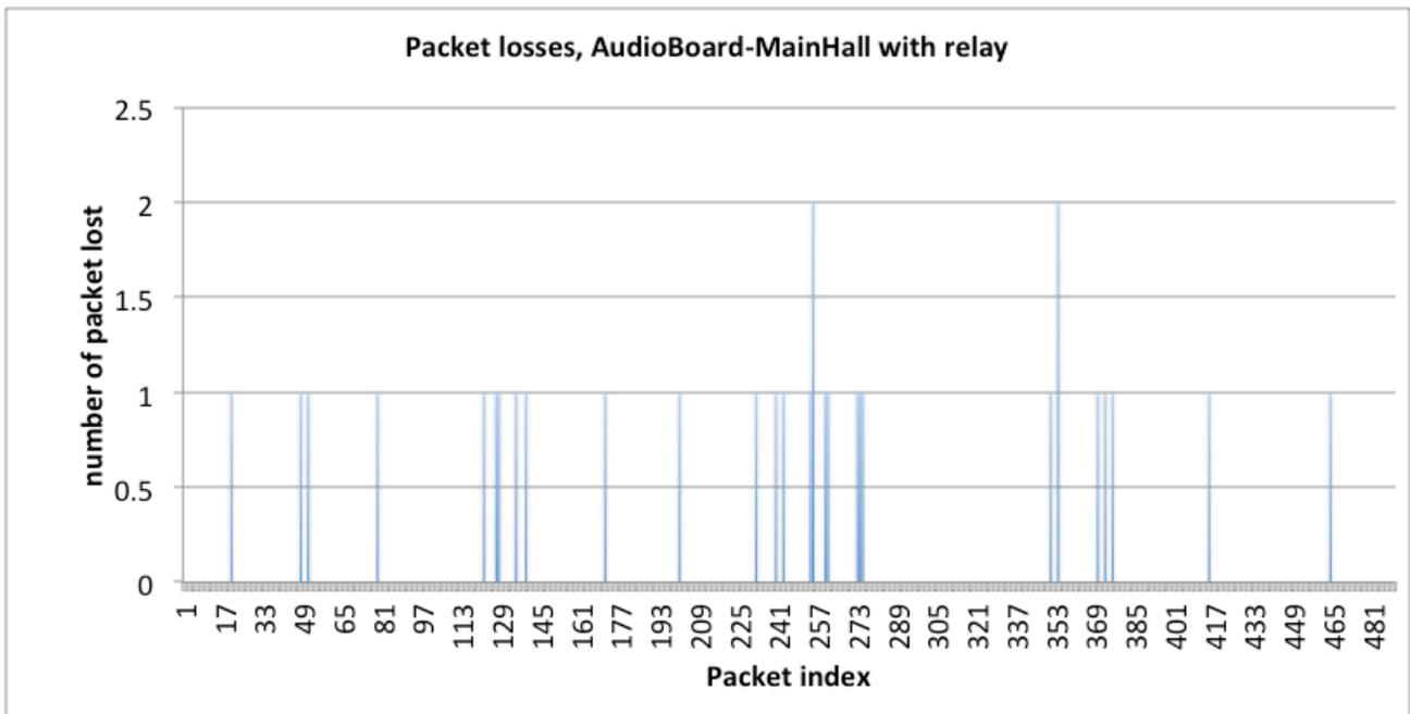
Figure 58 : number of lost packets in a row, A2 level, test#3
