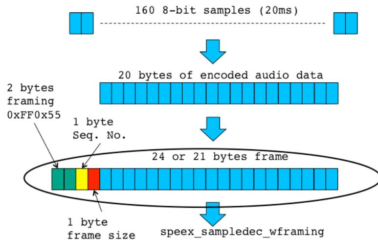
Figure 12: audio frame format, encoded audio data are in speex format
