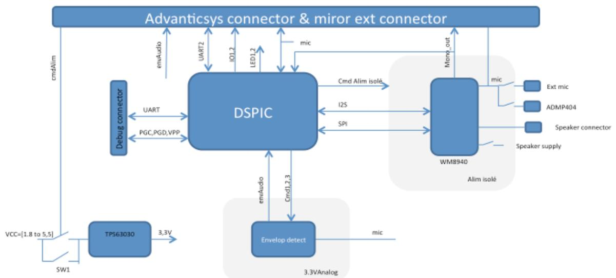
Figure 9: developed audio board schematic
