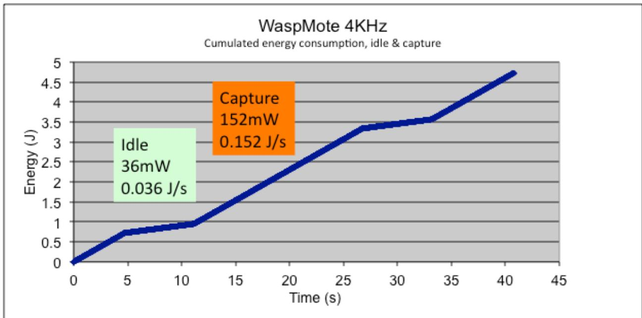
Figure 63: cumulated energy consumption, WaspMote audio, 4kHz, idle & capture
