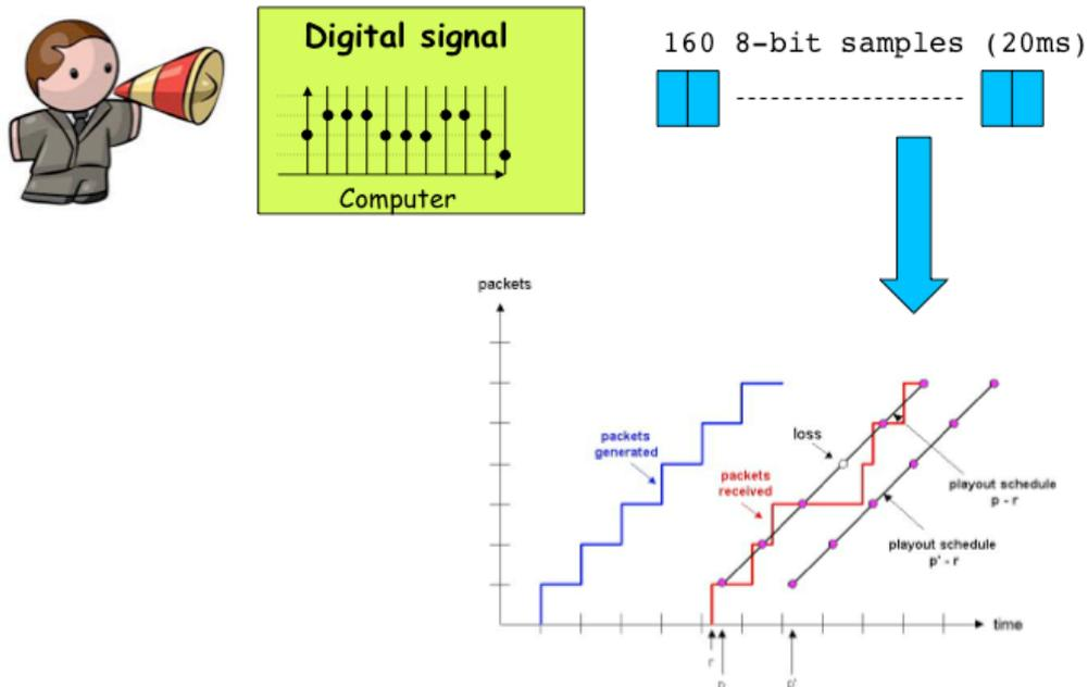
Figure 6: playout buffer to handle packet jitter
