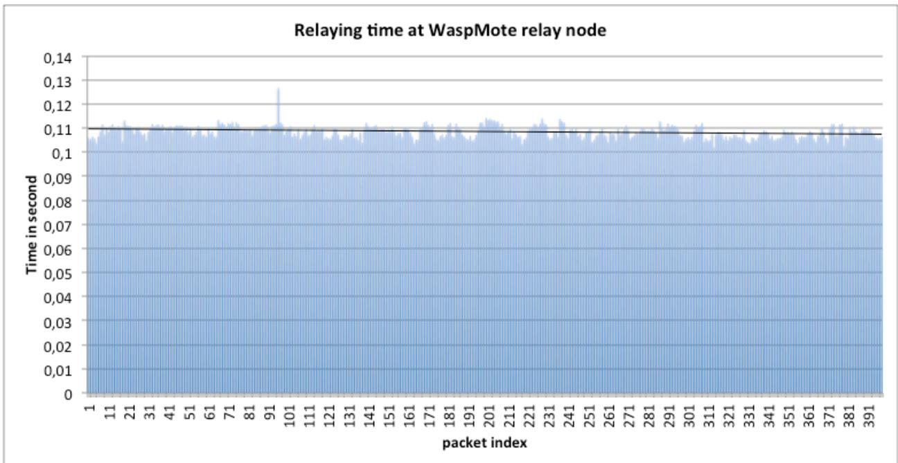
Figure 44 : relay time of the relay node, A6 level so 96-byte packet, test #10
