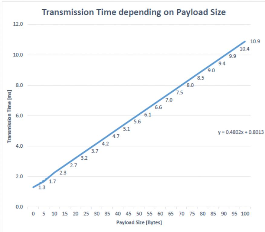
Figure 73 : TST mote sending overhead
