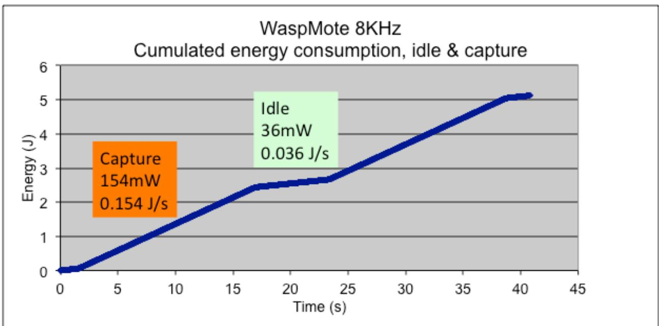
Figure 65: cumulated energy consumption, WaspMote audio, 8kHz, idle & capture
