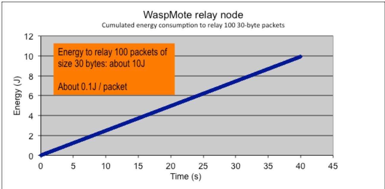
Figure 68: cumulated energy consumption WaspMote, relay
