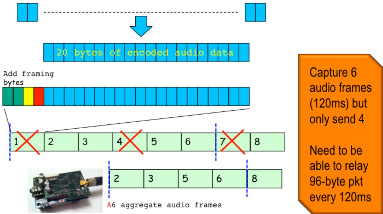
Figure 16: A6 aggregation mode for slow relay nodes
