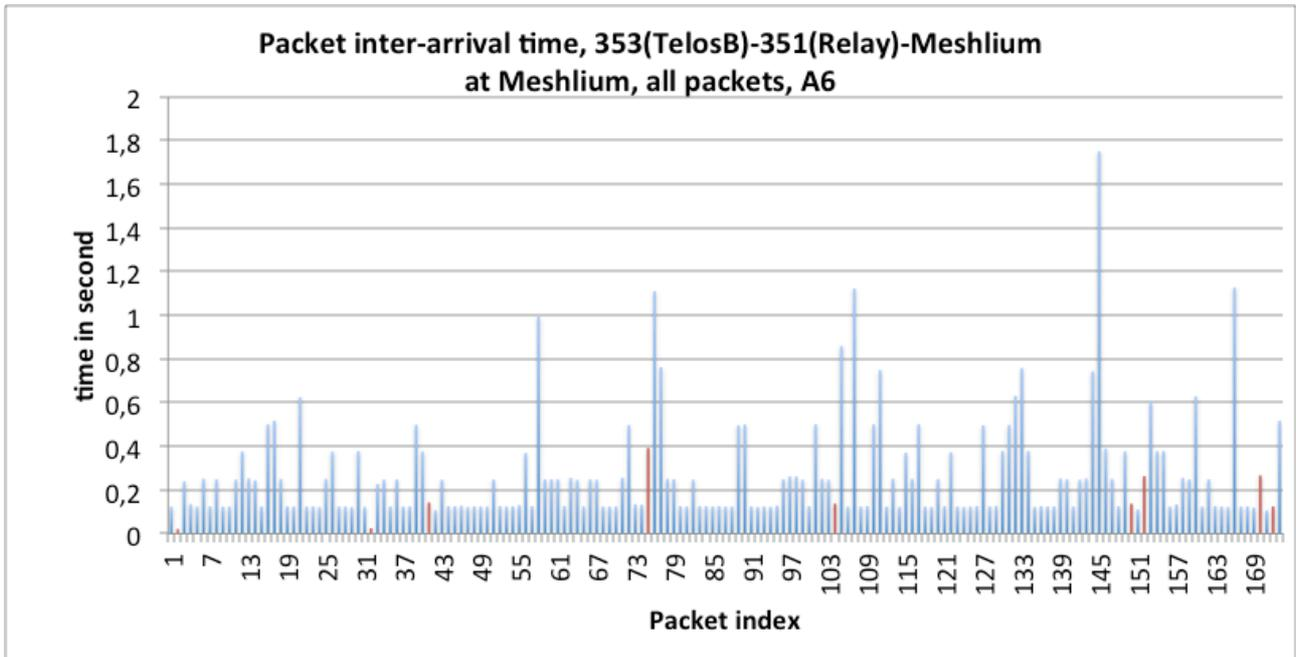
Figure 40 : packet inter-arrival time from both the audio source and the relay node, A6 level, test #9
