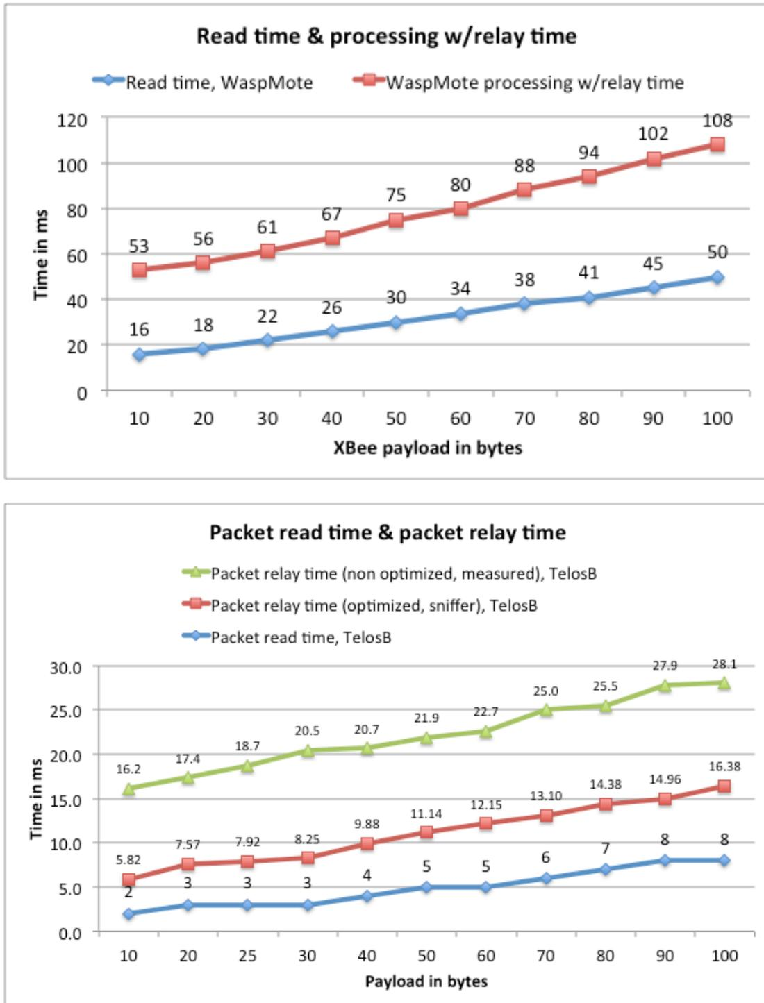
Figure 4:  $t_{read}$  and  $t_{relay}$  for WaspMote (top) and Advanticsys TelosB (bottom)
