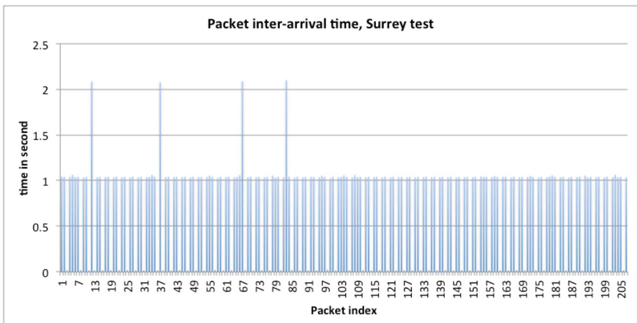
Figure 70 : packet inter-arrival time from the traffic generator, 100-byte packets
