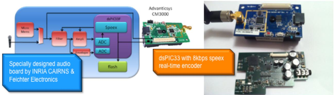
Figure 10: developed audio board and Advanticsys TelosB with the audio board
