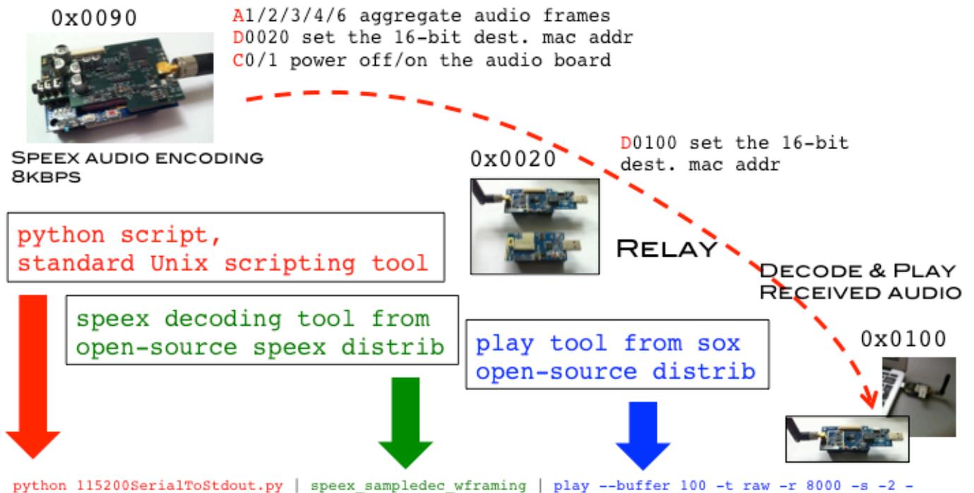
Figure 13: Multi-hop audio streaming scenario with the developed audio board
