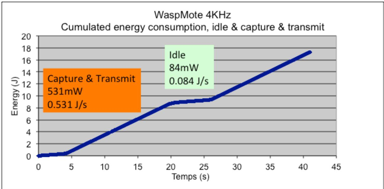
Figure 64: cumulated energy consumption, WaspMote audio, 4kHz, idle & capture & transmit
