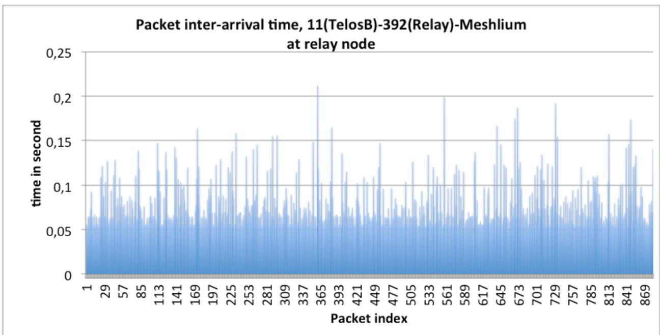
Figure 37 : packet inter-arrival time from the relay node, A1 level, test #4
