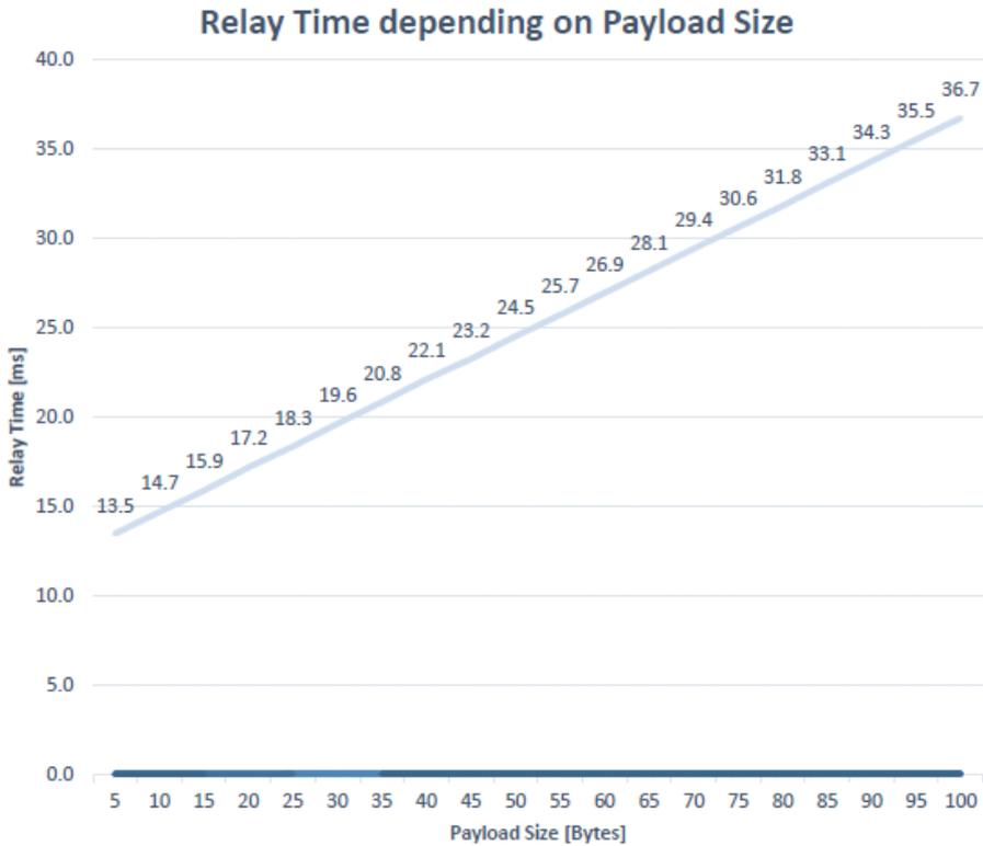
Figure 74 : TST mote relaying overhead
