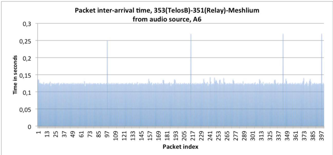
Figure 42 : packet inter-arrival time from the audio source, A6 level, test #10
