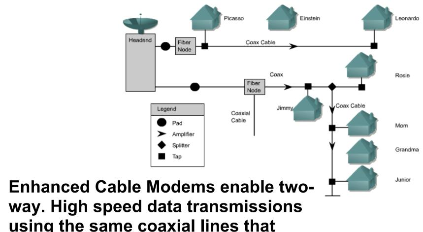
way. High speed data transmissions using the same coaxial lines that transmit cable television.
