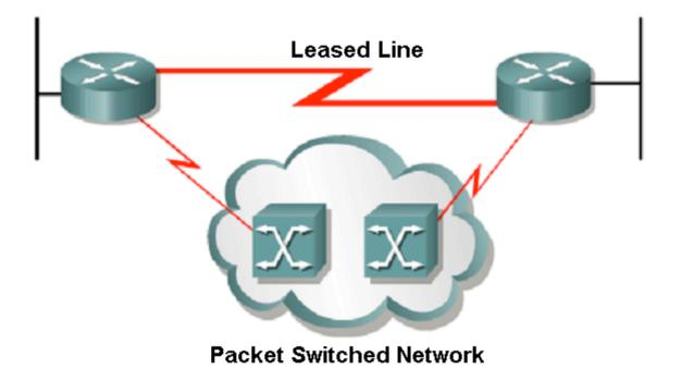
LANs can be connected with a long leased line or with shorter leased lines to a packet switched network. The packet network does the long haul.
