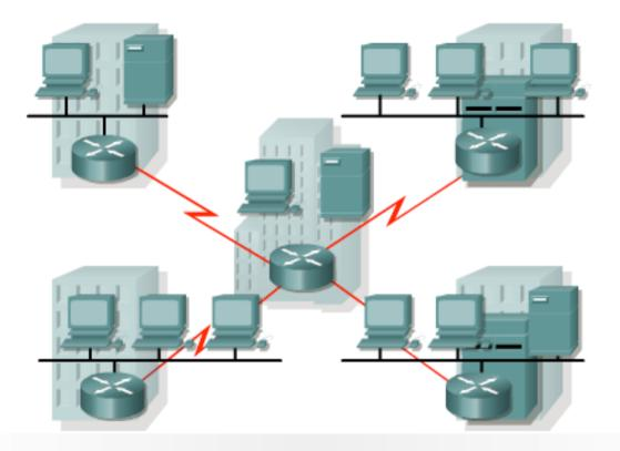
LANs separated by distance are linked by data communications lines and routers.
