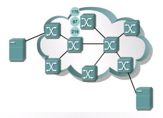
Labeled data is passed from switch to switch. It may have to wait its turn on a link.
