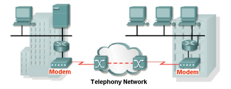
WAN built with intermittent connections using a modem and the voice telephone network.
