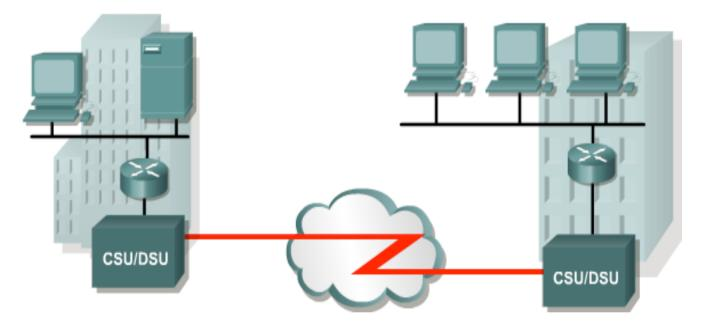
Leased lines are not only used to provide direct point-to-point connections between Enterprise LANS, they can also be used to connect individual branches to a packet switched network.
