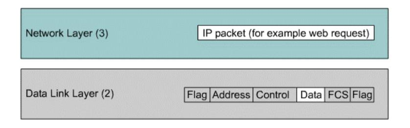
Network data is encapsulated in an HDLC frame.
