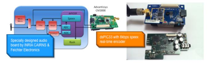
Figure 10: developed audio board and AdvanticSys TelosB with the audio board
