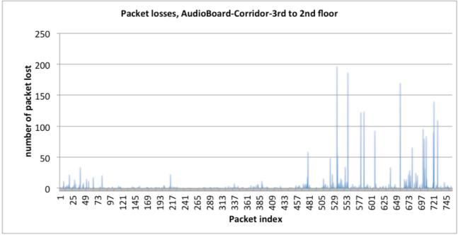
Figure 55 : number of lost packets in a row, A1 level, test#6
