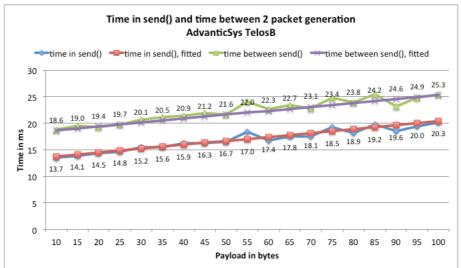
Figure 3: t<sub>send</sub> and t<sub>pkt</sub> for for WaspMote (top) and AdvanticSys TelosB (bottom)
