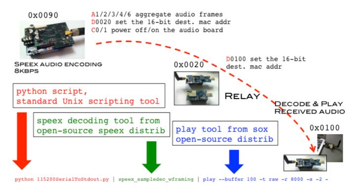
Figure 13: Multi-hop audio streaming scenario with the developped audio board
