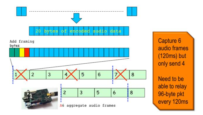
Figure 16: A6 aggregation mode for slow relay nodes
