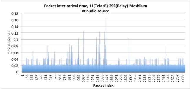
Figure 36 : packet inter-arrival time from the audio source, A1 level, test #4
