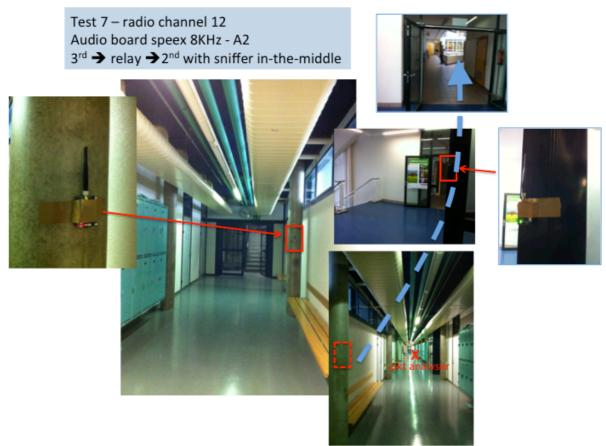
*Figure 59 : test#7 in a long corridor of the HEPIA building, receiver in 2nd floor, relay at corridor entrance, near the stairways*
