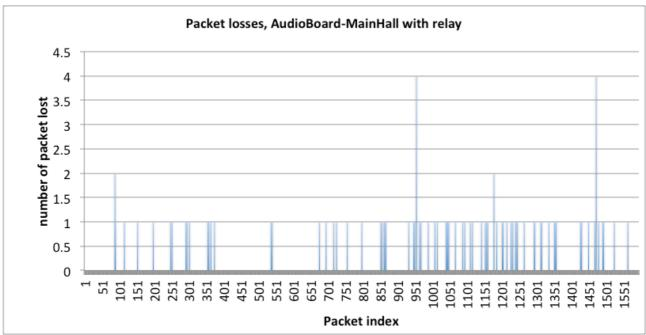
Figure 57 : number of lost packets in a row, A1 level, test#2
