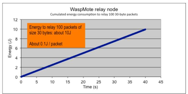
Figure 68: cumulated energy consumption WaspMote, relay
