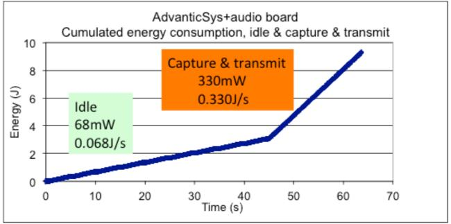
Figure 67: cumulated energy consumption AdvanticSys TelosB+audio board, idle & capture & transmit
