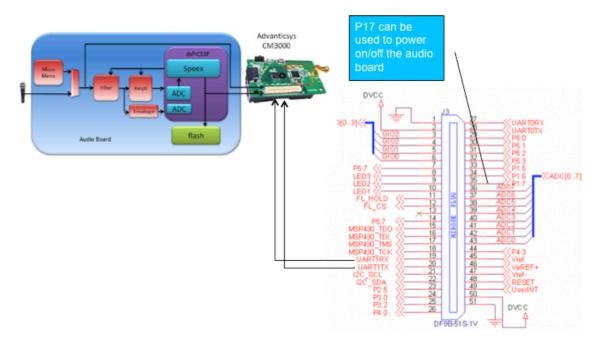
Figure 11: developed audio board connectivity schema on an AdvanticSys TelosB
