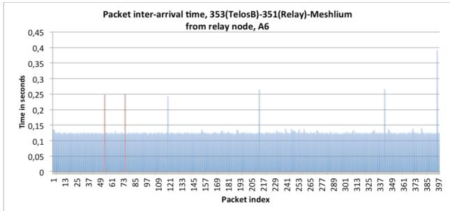
Figure 43 : packet inter-arrival time from the relay node, A6 level, test #10
