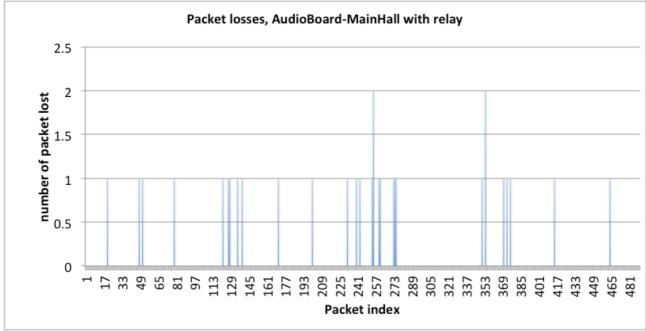
Figure 58 : number of lost packets in a row, A2 level, test#3
