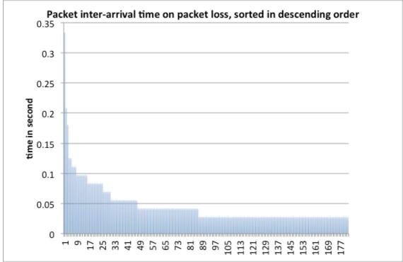
Figure 28 : packet inter-arrival time after losses, test #6. First ON period, descending order.
