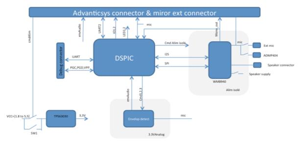
Figure 9: developed audio board schematic
