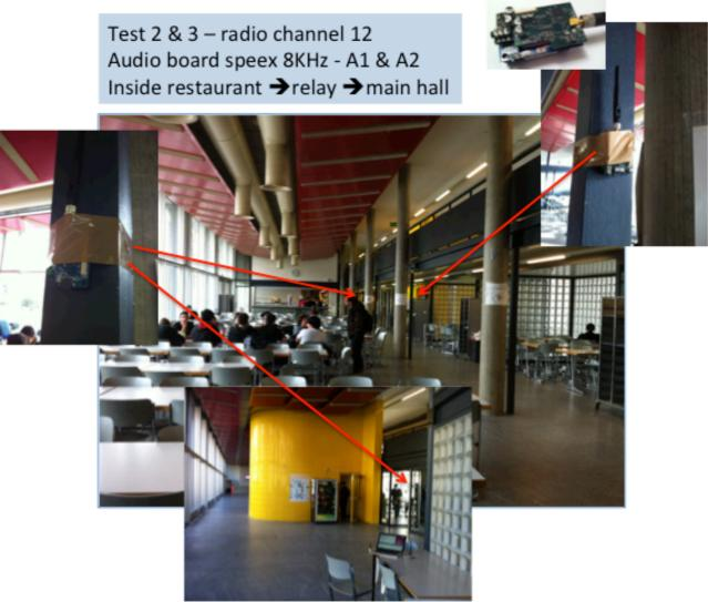
Figure 56 : test#2 & test#3 in the main hall of the HEPIA building, with relay node
