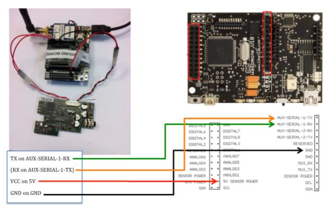
Figure 72 : connecting the audio board to a Libelium WaspMote
