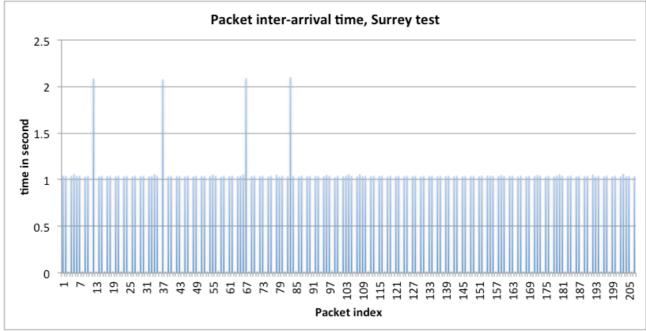
Figure 70 : packet inter-arrival time from the traffic generator, 100-byte packets
