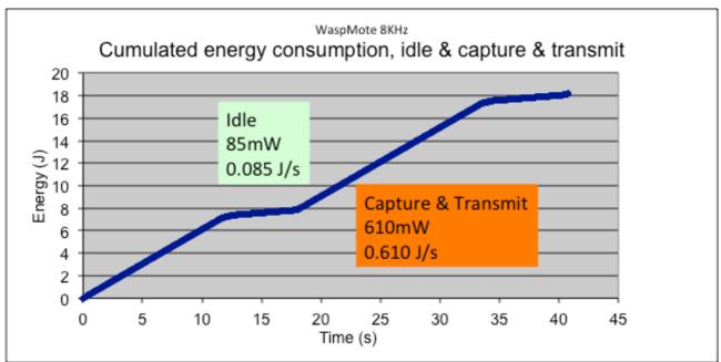
Figure 66: cumulated energy consumption, WaspMote audio, 8kHz, idle & capture & transmit
