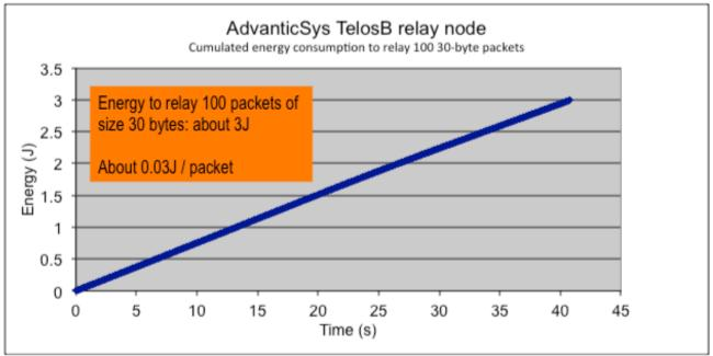
Figure 69: cumulated energy consumption AdvanticSys Telosb, relay
