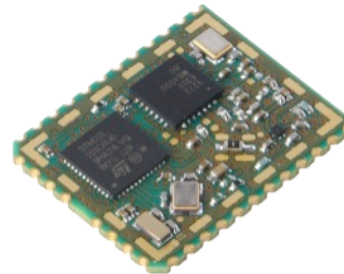
IMST IM880A-L is based on Semtech SX1272 LoRa 863-870 MHz for Europe
