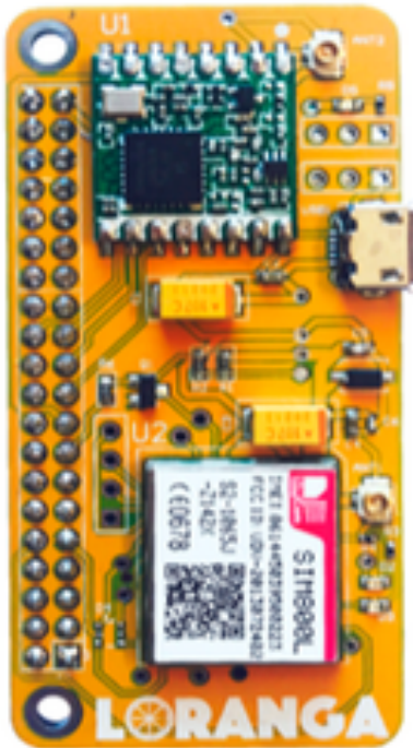
LORANGA LoRa + 2G/3G board, mainly for Raspberry Pi
