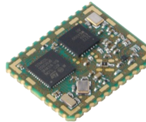
IMST IM880A-L is based on Semtech SX1272 LoRa 863-870 MHz for Europe
