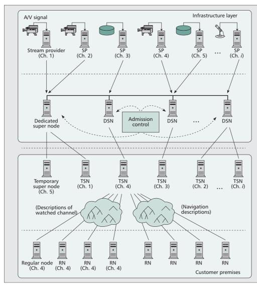
In P2P networks, there are two main approaches to video distribution: tree and mesh. The tree approach, based on multicasting on the application layer, has a distribution structure always ready for transmission. The mesh approach employs connections on demand.
