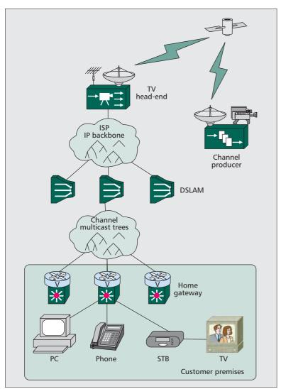
Figure 2. Typical commercial IPTV architecture.
