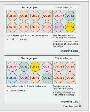
Figure 4. Utilization of the user bandwidth in each viewing state for the prejoin schemes proposed in [2].
