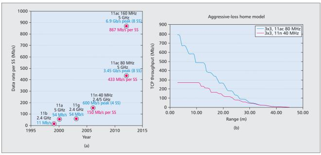
Figure 1. a) Peak data rate and the per-spatial stream (SS) data rate of WLAN technologies; b) rate-over-range of three spatial stream 802.11ac and 802.11n devices.
