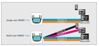
Figure 3. Illustration of MU-MIMO 802.11ac and SU-MIMO 802.11n.
