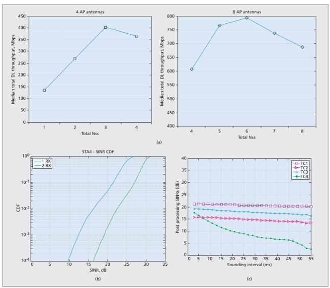
**Figure 5.** a) Median throughput vs. total number of MU-MIMO spatial streams (Nss) across all STAs; b) CDF of MU-MIMO post-processing SINRs with 1 Rx antenna and 2 Rx antennas (interference nulling enabled); c) MU-MIMO post-processing receiver SINRs, over time, for different user test cases (TC): TC1 — watching a movie; TC2 — typing on the keypad; TC3 — holding the device to the ear; TC4 — walking.
