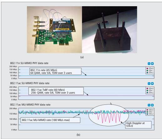
Figure 4. a) 4 × 4 802.11n mini-PCIe card and MU-MIMO access point; b) time snapshot from OTA MU-MIMO prototype in LOS, high SNR scenario.
