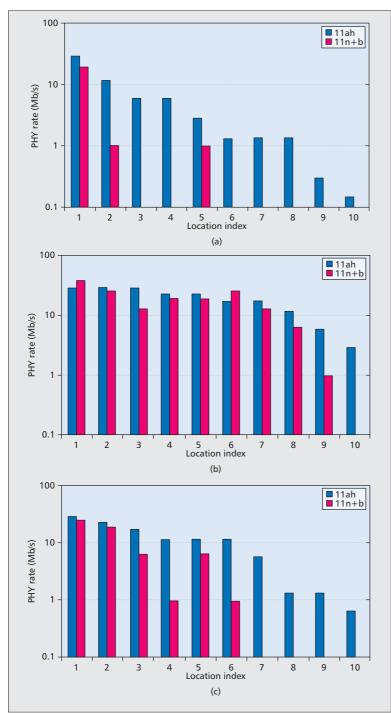
**Figure 6.** Rate and coverage advantage of 802.11ah over 802.11n and 802.11b in single-family homes: a) 2230 ft<sup>2</sup> home with basement and yard space (2.4 GHz path losses: 76–104 dB); b) 3500 ft<sup>2</sup> single-family home with two floors (2.4 GHz path losses: 72–94 dB); c) 4249 ft<sup>2</sup> home with basement, backyard, and front yard (2.4 GHz path losses: 76–98 dB).
